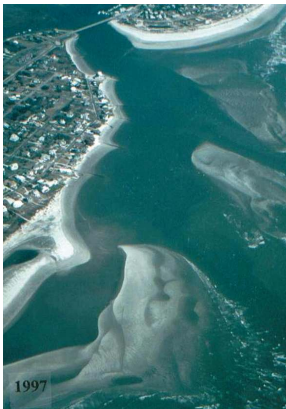
FIGURE 16. Artificial structures (such as seawalls, groins, and jetties) are used to anchor parts of the coast, often with negative as well as positive effects. In some settings, their impacts are dwarfed by natural features like the inlet bar (in the foreground), which is acting as a natural breakwater. Sullivan's Island, SC, USA
