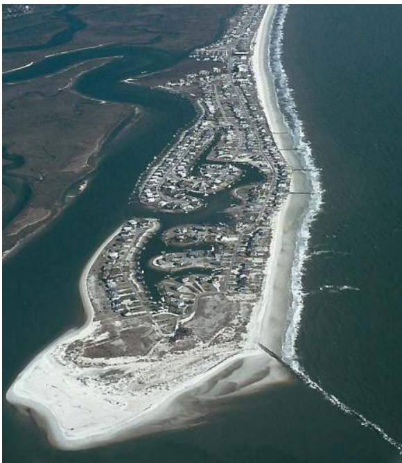
Garden City (SC) – Groins (center of image) were placed to counter focused erosion along the bulge left from a former inlet.
