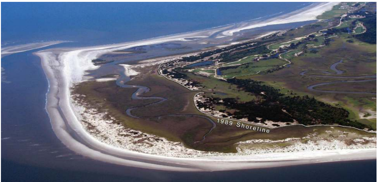
FIGURE 22. The eastern end of Kiawah Island (SC) (2008) where shoal-bypassing events between 1990 and 2005 added 5 million cubic yards to the island and created a 3-mile-long barrier beach and lagoon system. Episodic events such as this illustrate how rapidly barrier islands can form in the presence of an ample sediment supply. [Source: CSE 2009]
