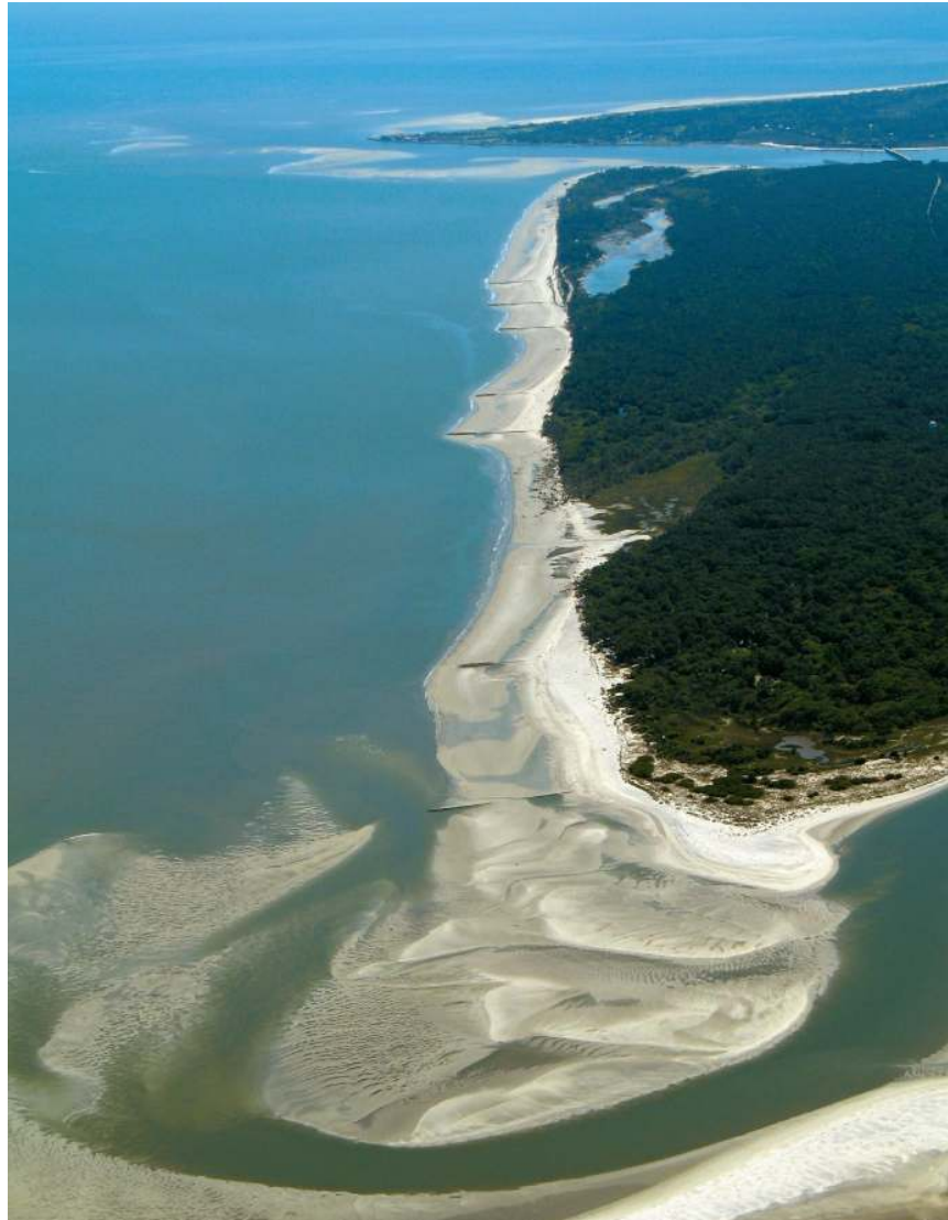
Hunting Island (SC) at low tide in April 2010 after eight nourishment projects (1968–2006) and construction of six groins (2007) designed to retain sand along segments of the 6.5-kilometer-long (4 miles) barrier island. Few sites have posed greater challenges for beach restoration, given Hunting Island's historical erosion rate of ~8 meters (~25 feet) per year. [See Traynum et al (2010) for a summary of shore-protection measures and the semi-soft solution CSE designed for the island.]
