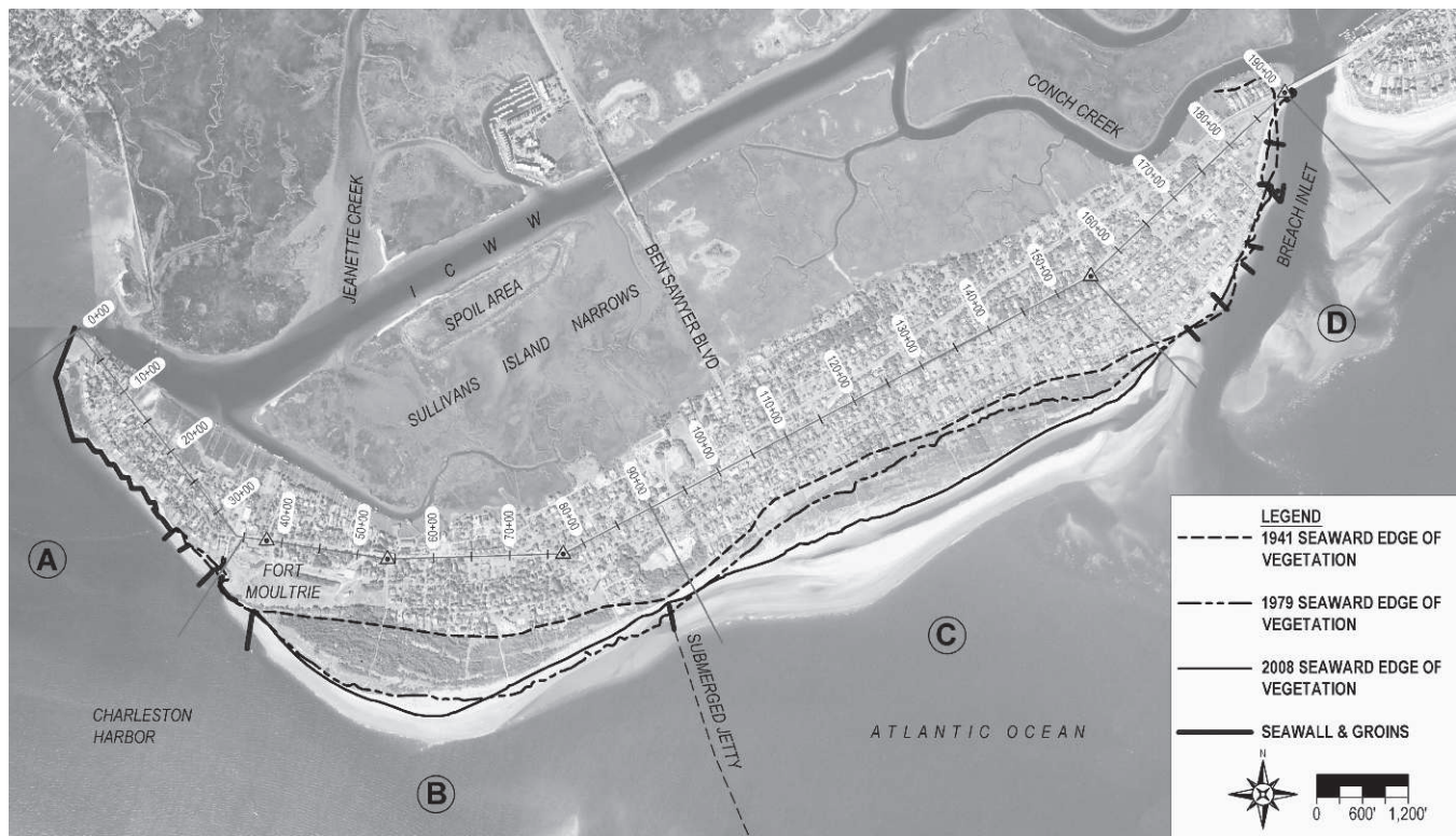
Figure 16. Shoreline change along Sullivan's Island 1941–2008 superimposed on a 2008 image (courtesy South Carolina Department of Natural Resources).
