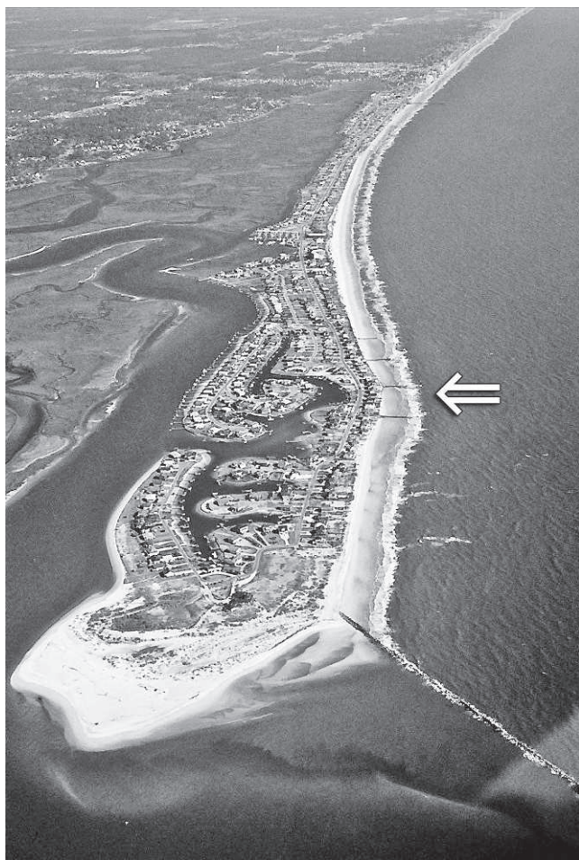
Figure 10. Murrells Inlet and Garden City looking north in 1987. Collapsed shoals of a former inlet from the early 1900s produced a salient (arrow) which has been a focal point of erosion and shore protection measures during the past 50 years.
