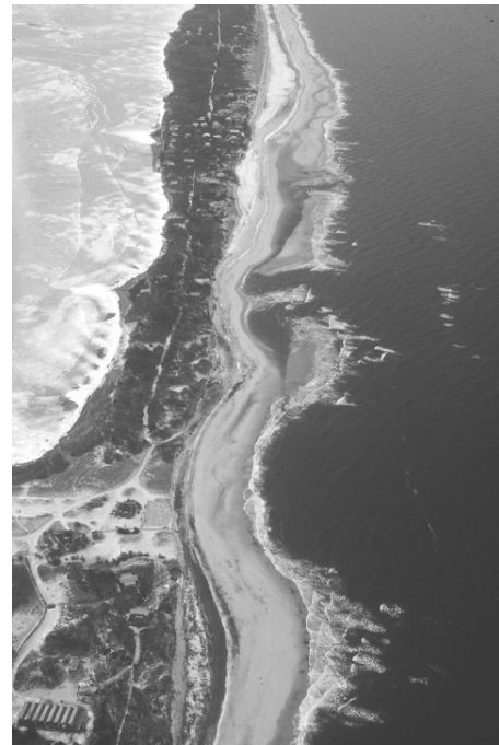
Figure 6. Oblique aerial photograph at low tide on 11 January 1994 showing rhythmic shoreline features along a section of central Fire Island. The partially attached low-tide bars (center, right side of image) are estimated to contain no more than 50 \text{ m}^3/\text{m} . (Photo by T.W. Kana)
