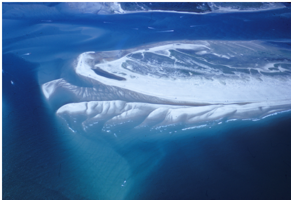
Figure 9. Oblique aerial photo of Monomoy Island (MA) spit at low tide (circa 1970) showing trailing, ebb-tidal delta shoals welding to the updrift beach. This process is considered analogous to spit growth at western Fire Island between 1825 and 1940, prior to jetty construction. (Source photo: Courtesy of Miles O. Hayes, Research Planning, Inc.)
