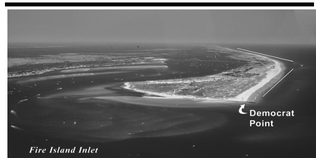
Figure 4. Oblique aerial photograph at low tide in August 1981 looking east at Fire Island Inlet. The ~1,500-m-long jetty at Democrat Point was constructed in 1940 and filled to capacity by the mid-1950s (Saville, 1961). The 2-km-long fillet associated with the jetty is oriented east-west, a difference of ~17° from the azimuth of central Fire Island. (Photo by T.W. Kana)
