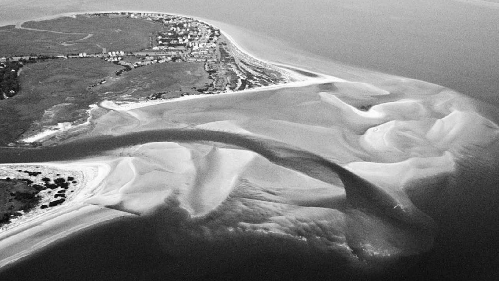
Figure 3. Oblique aerial photo at low tide on 10 February 2006, showing the exposed shoals of the Johnson Creek ebb-tidal delta which is estimated to contain ~20 million cubic yards. The northern spit of Hunting Island is at the lower left. A terminal groin was constructed at the end of the spit in 1969.
