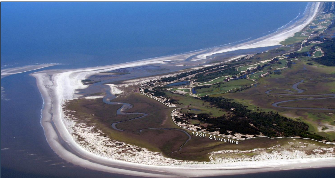
Kiawah Island SC USA—The eastern end of the island (2008) where shoal-bypassing events between 1990 and 2005 added 5 million cubic yards to the island and created a 3-mile-long barrier beach and lagoon system. Episodic events such as this illustrate how rapidly barrier islands can form in the presence of an ample sediment supply. [Source: CSE 2009]
